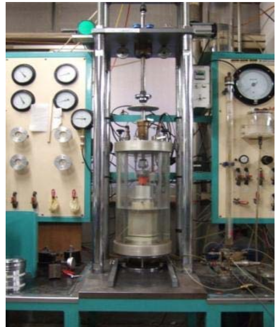
Photo. 3. Hollow-cylindrical torsional test apparatus
