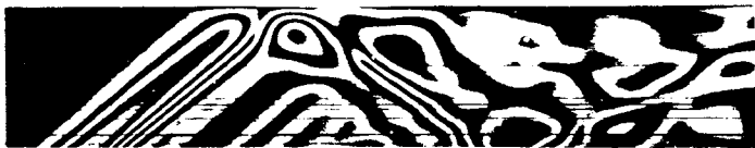
Fig. 3 Streak photography of photoelastic fringe pattern, incident P wave, \phi=7
