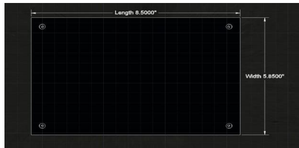
Figure 21: Upper part of the wafer box (Auto CAD 2D plan view)
