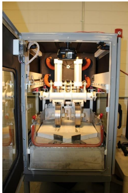
Figure 13: Advanced Pavement Analyzer inside arrangement (APA) Jr.
