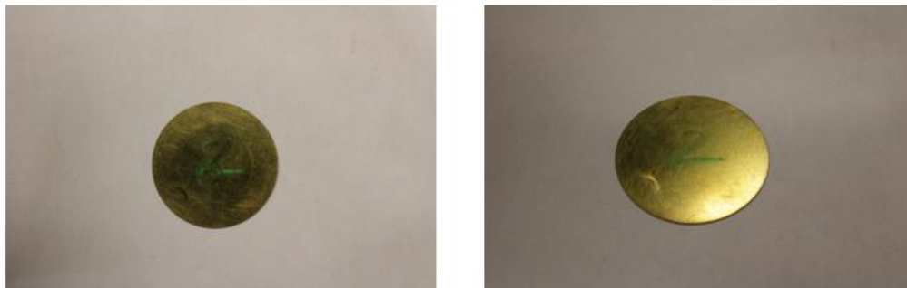
Figure 18: Piezoelectric sensor used to harvest energy (Bottom view)
