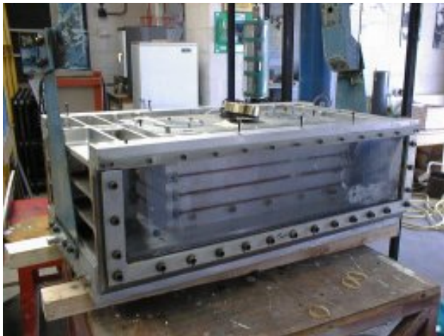
Fig. 10. Equivalent Shear Beam (ESB) container (Thusyanthan et al., 2007).
