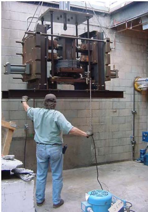
Fig. 3. Large-diameter CyDSS apparatus (currently at Arizona State University).
