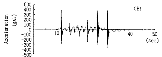
Fig.4 Acceleration history of base motion at location CH1
