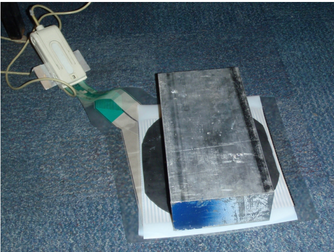
Fig. 8 Direct shear test set-up.
