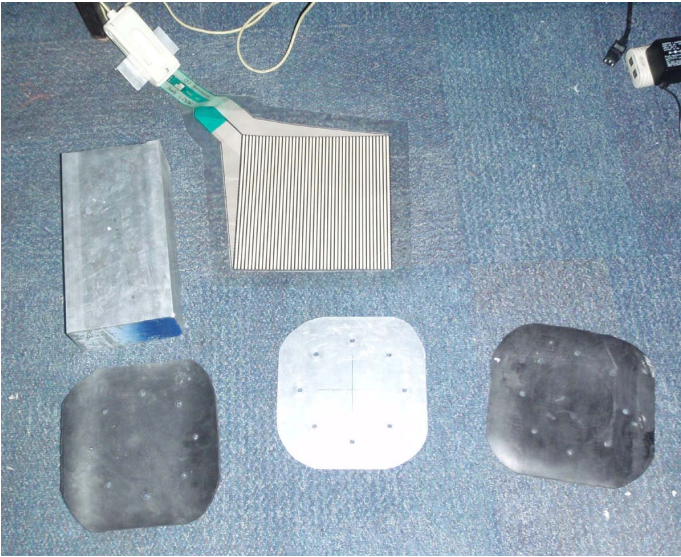
Fig. 7 Two rubber mats, thin aluminum plate, thick aluminum block, and a tactile pressure sensor used in direct shear tests.
