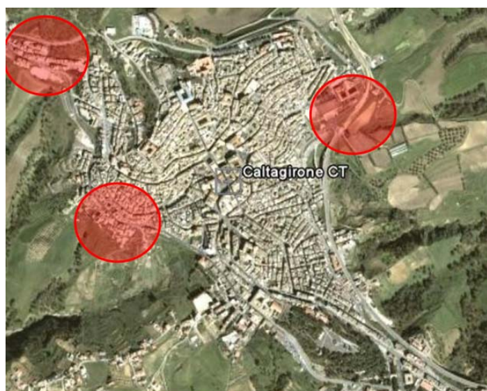
Fig. 4: An aerial photo of Caltagirone: the most landslide prone areas are evidenced.
