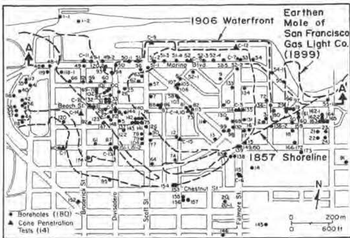
Figure 2. Locations of Conventional Boreholes, Cone Penetration Soundings, and Cross-Section A-A' in the Marina District
