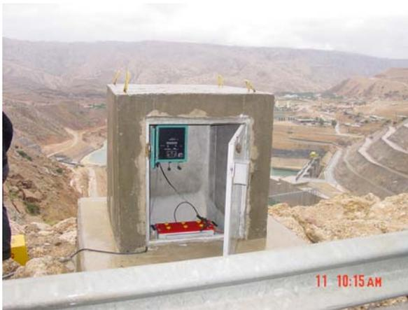
Fig.3. the located accelerometer on the crest
