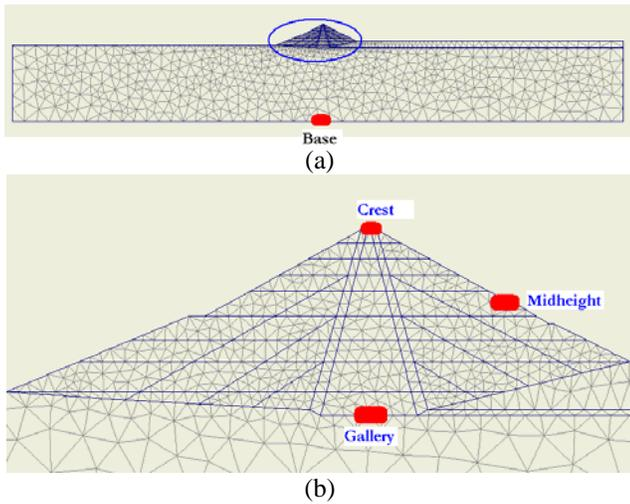
Fig.2. the 2-D mesh of the Masjed Soleiman dam body and the considered foundation and also the location of accelerometers, (a) general view, (b) a more coarse view of dam body
