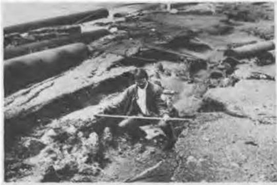
Fig. 2 Typical ground surface manifestations of soil liquefaction
