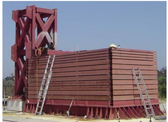
Fig. 4. Soil container and reaction tower
