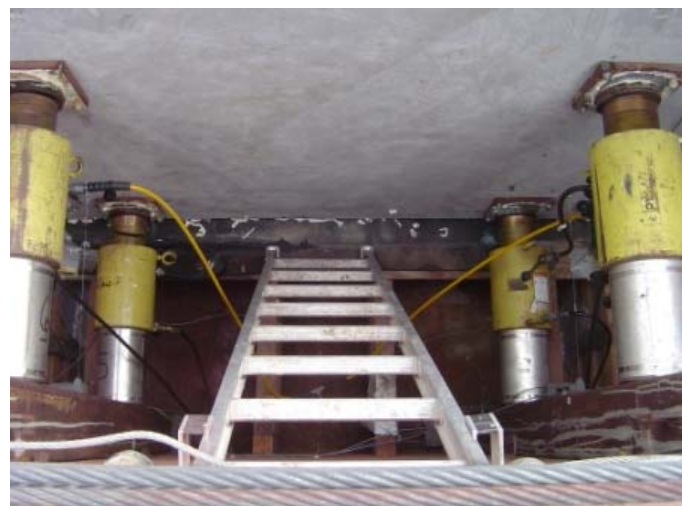
Fig. 6. View looking down at extended plunger jacks reacting against load cells behind test wall
