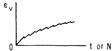
Fig.1. Total residual compression strain after Nth cyclic loading.
