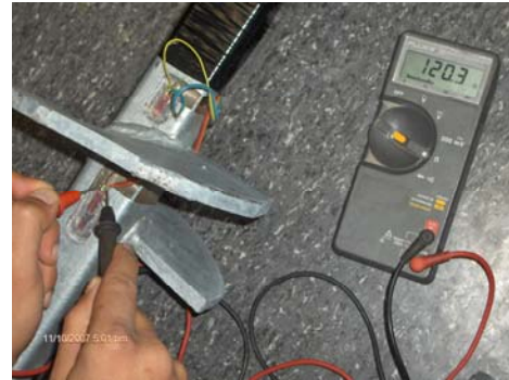
Fig.5. A Pair of strain gauges installed and the resistance of the strain gauge is measured with an Ohm-meter
