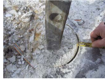
Fig.17. FRP-G-HSP with external grout – separation between the FRP tube and the external grout during lateral testing
