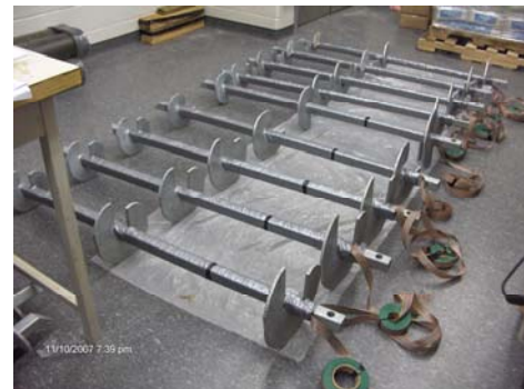
Fig.6. Finished instrumented lead sections
