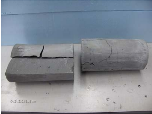
Fig.2. Splitting tensile strength test on the cylinders without (left) and with steel fibres (right).
