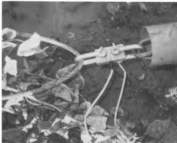
Fig. 11 Explosive tie allowing a sudden tension release.
