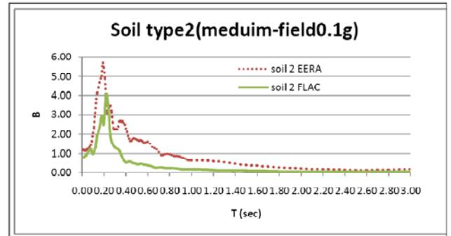
Fig. 9. Acc. Response Spectra through linear and nonlinear approaches in soil type 2 (medium field)
