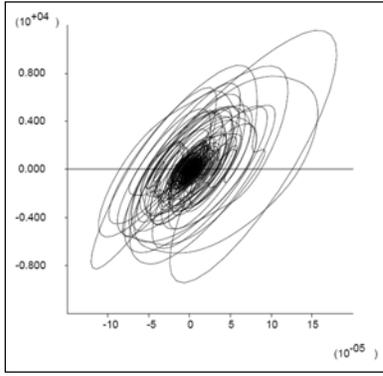
Fig. 15. The hysteresis stress-strain loops of soil 2 obtained in *FLAC*
