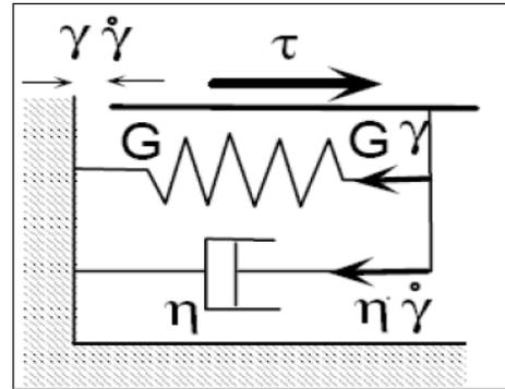
Fig. 2. Schematic representation of stress-strain model used in equivalent-linear model
