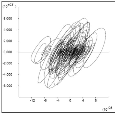
Fig. 16. The hysteresis stress-strain loops of soil 3 obtained in *FLAC*
