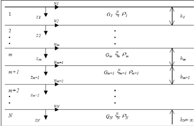
Fig. 1. One-dimensional layered soil deposit system (after Schnabel et al., 1972).
