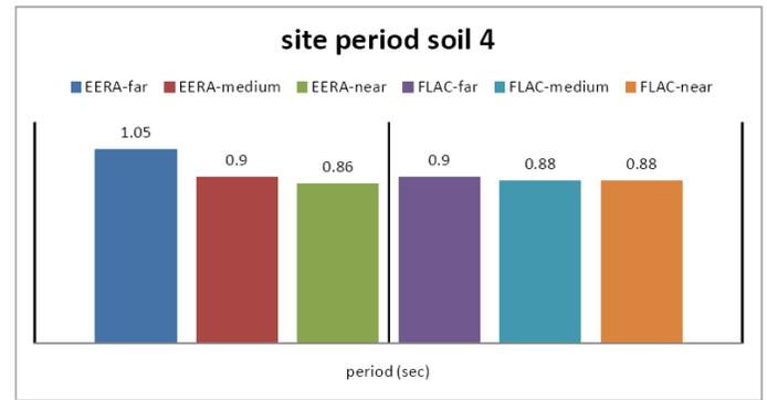
Fig. 14. Comparison of natural site period by linear and nonlinear approaches in soil type 4
