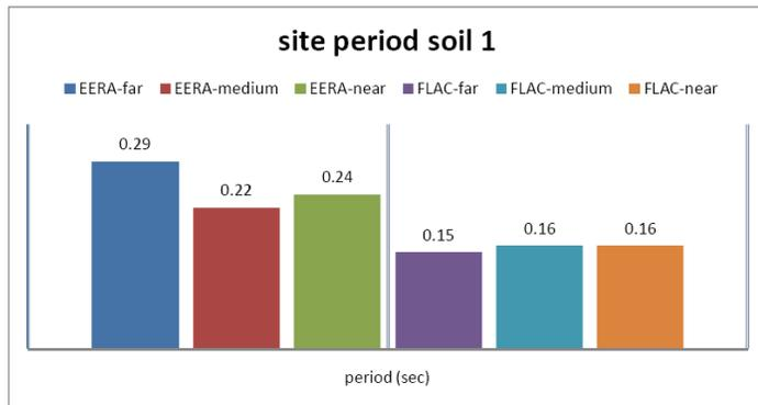
Fig. 11. Comparison of natural site period by linear and nonlinear approaches in soil type 1
