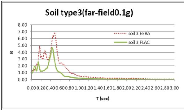
Fig. 6. Acc. Response spectra through the linear and nonlinear approaches (under Eq. Chichi-Taiwan).
