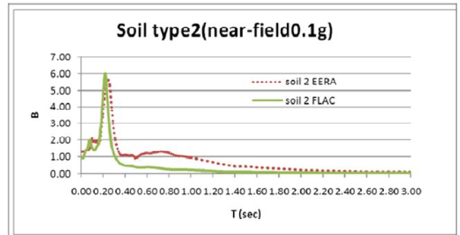
Fig. 10. Acc. Response Spectra through linear and nonlinear approaches in soil type 2 (near field)
