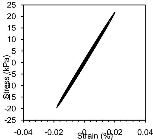
Fig. 17. The hysteresis stress-strain loops of soil type 3 obtained in *EERA*
