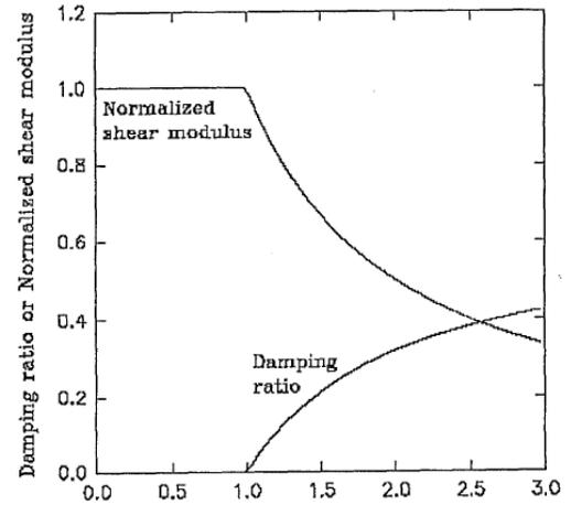
Fig. 4. Modulus and damping ratio versus cyclic strain for the elastoplastic model FLAC
