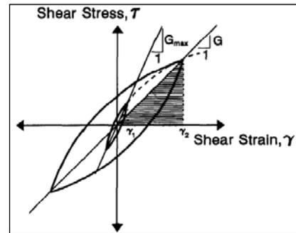
Fig. 3. Equivalent-linear model, hysteresis stress-strain curve
