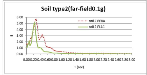
Fig. 8. Acc. Response Spectra through linear and nonlinear approaches in soil type 2 (far field)
