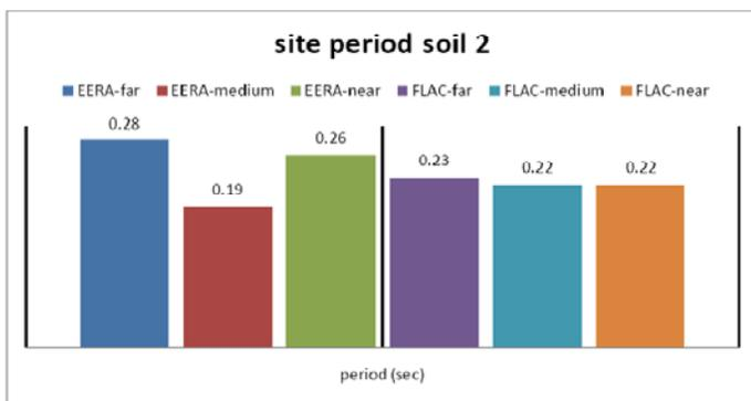
Fig. 12. Comparison of natural site period by linear and nonlinear approaches in soil type 2
