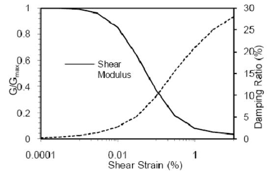
Fig. 5. The Modulus ratio and damping curves used in the equivalent-linear model
