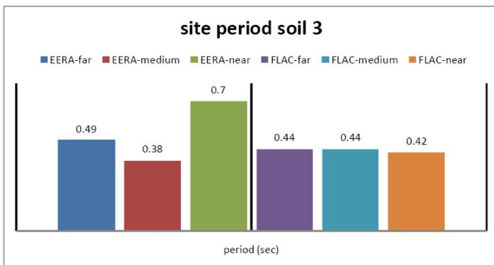
Fig. 13. Comparison of natural site period by linear and nonlinear approaches in soil type 3
