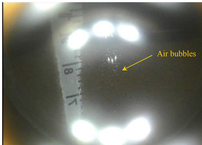
Photo 2. Existence of air bubbles after shaking test
