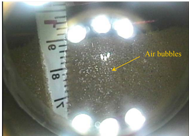
Photo 1. Existence of air bubbles before shaking test
