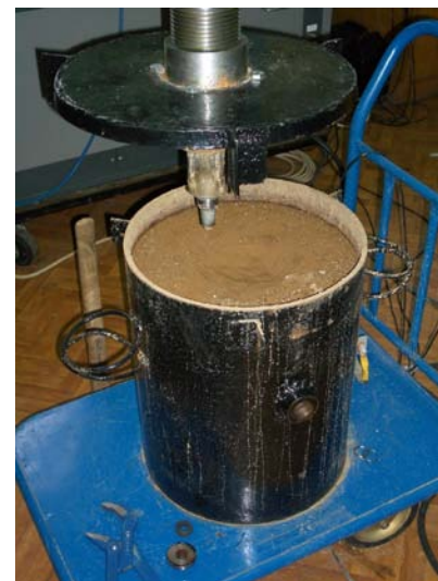
Fig. 3. Test box, filled with water-saturated sand.
