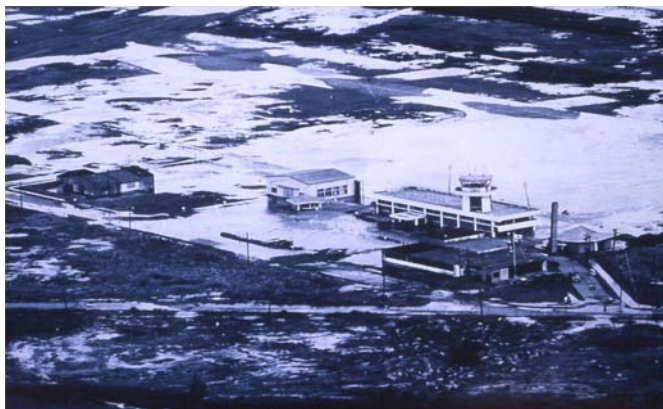
Fig. 27. Boiled water around Niigata Airport (air photograph taken by Mr. Yuminamochi immediately after the quake).
