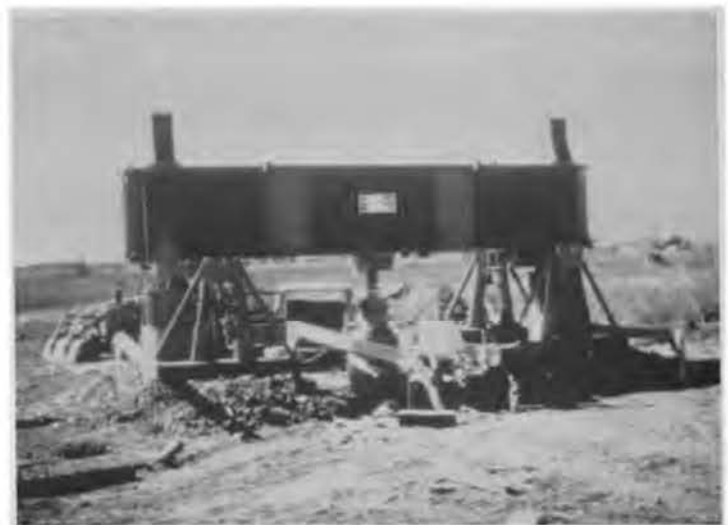
FIGURE 6 - Pile Load Tests, TAMU Clay Site
