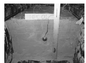
Fig. 8. Geotechnical centrifuge model test: (a) model with instrument layout for in-flight condition; (b) before shaking; (c) soil dissection after shaking. The final positions of the target objects from model dissection after the centrifuge testing are also shown in (a) (M1' ~ M6').
