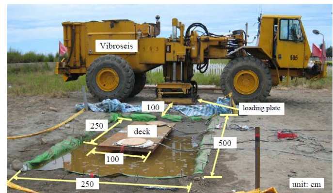
Fig. 2. Vibroseis truck and setup of wharf model test
