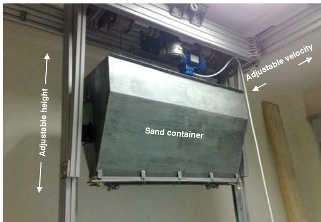
Fig. 5. Sand raining system used for model preparation.
