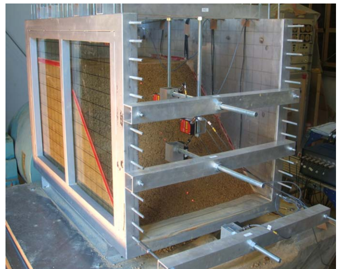
Fig. 4. Overview of slope model after construction.
