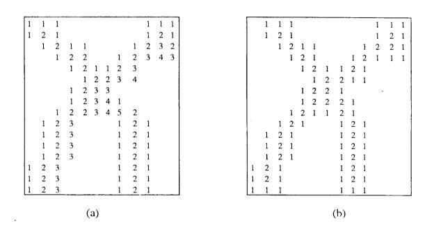
Fig.3. a. Distance values of pixels after first passb. Distance values of pixels after second pass
