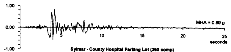
Figure 9(b): Acceleration time history recorded at a near-field soil site (instrument corrected data from CSMIP, 1994).
