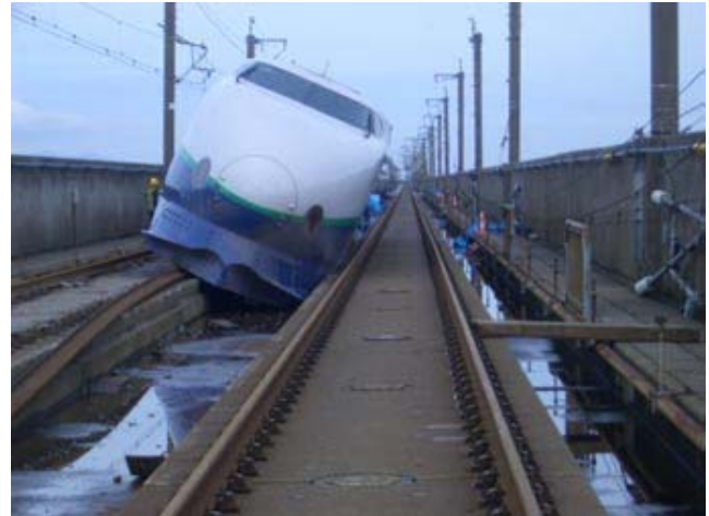
Figure 32: Derailed Shinkansen (Oct. 31) (photo: C. Scawthorn).
