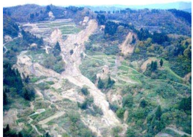
Figure 25: Typical debris flow, exhibiting a narrow path and long runout.
