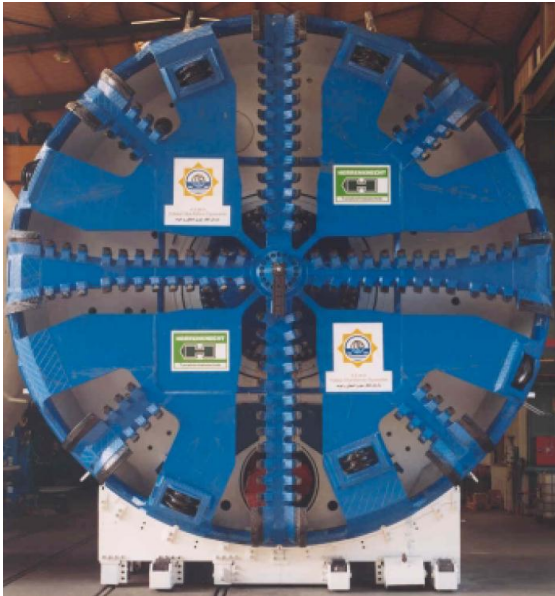
Fig. 2. EPB/TBM employed for Esfahan subway project
