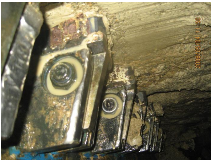
Fig. 3. Cutting Knife bits with carbide inserts
