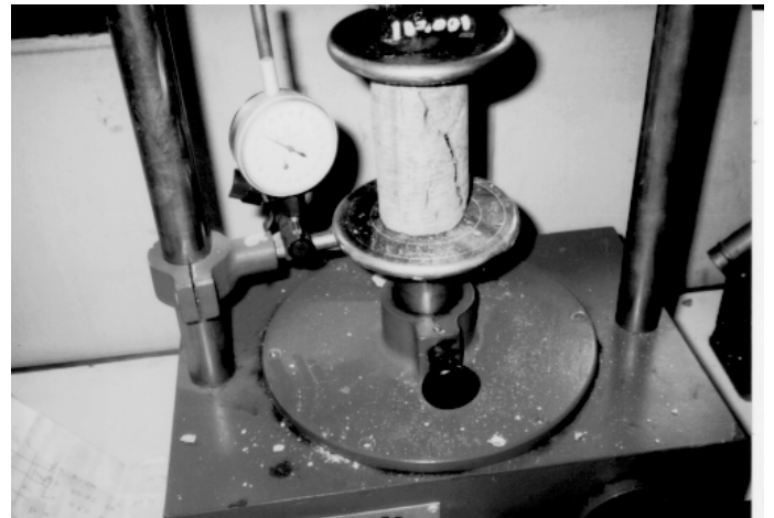
Fig. 9. Unconfined compression test of jet grouted sample.
