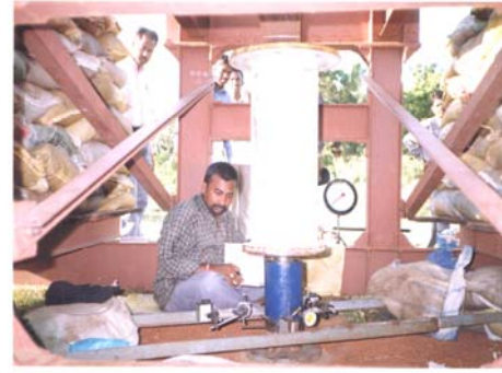
Fig.4 Experimental set-up for conducting Cyclic Load Test
