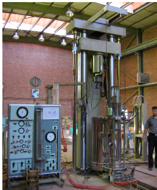
Fig. 1: Cyclic triaxial testing facility at BHRC
