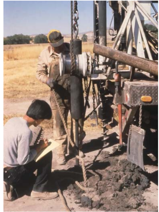
Fig 11. Student recording raw blow counts from a SPT test at Hamilton Field study site, along north shore of San Francisco Bay. Students were required to calculate the appropriate corrections years before industry routinely employed such practice.
