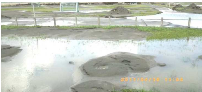
Fig. 2. Liquefied sand and sand ejection in front of distorted Tone river levee (Towhata et. al 2011)
