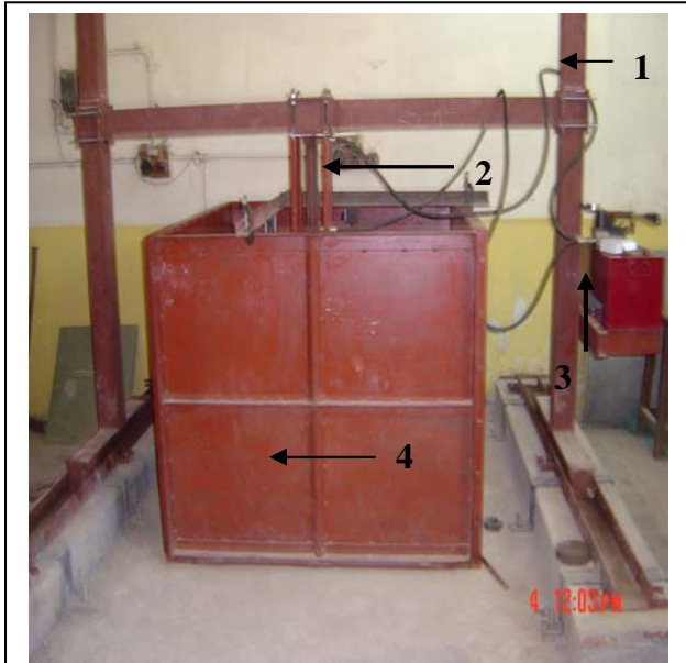
1: Loading Frame 2: Hydraulic Jack 3: Hydraulic Pump 4: Model Testing Tank
