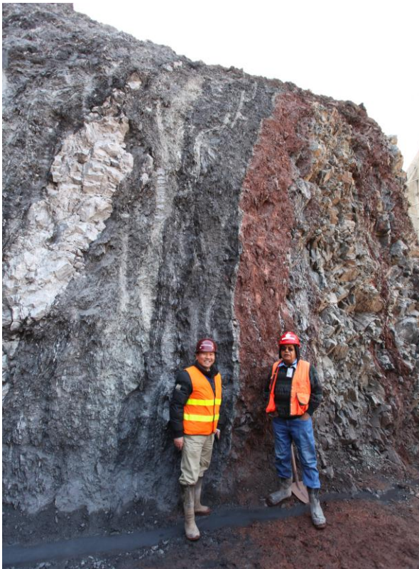
Fig. 3. Main Boundary Thrust, faulted contact Panjal Fm (left) and Murree Fm (right)
