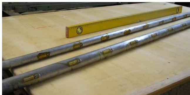
Fig.2 Appearance of piles equipped with strain gauges
