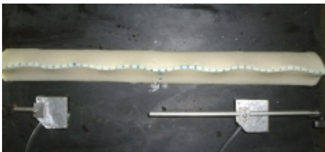
Fig.5. Photograph of embankment during the shaking
