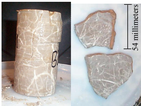
Fig. 7. Calcite filling fractures and fissures of intact rock controlling the plane of failure
