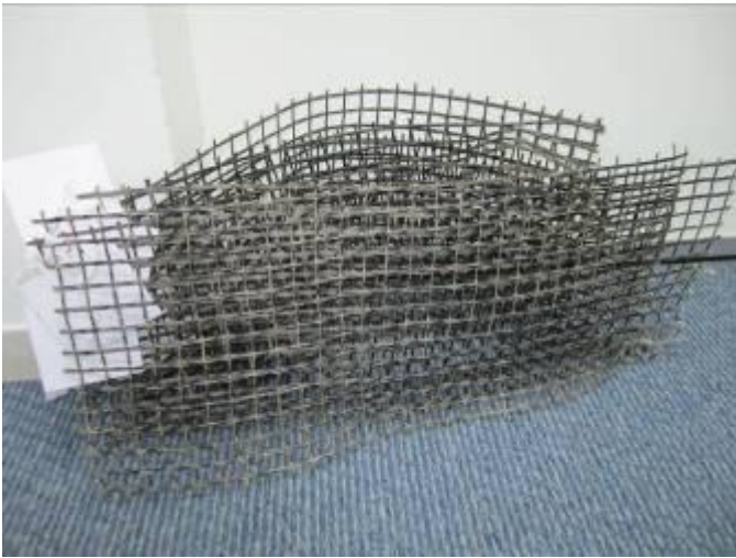
Fig.23. Samples of geogrid with minimum size of 600mm (Wrap) by 200mm (Weft) ready to send to an accredited laboratory
