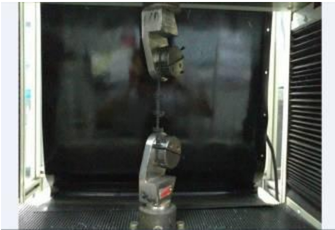
Fig. 24. Wide Width Tensile Test using split roller grips based on ISO 10319-2008
