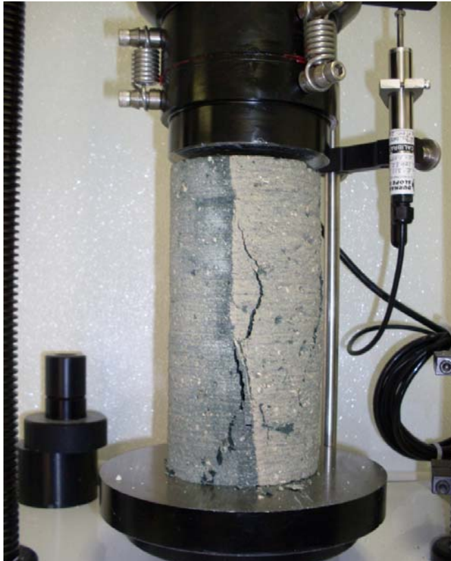
Fig. 12. Core Sample at Joint
