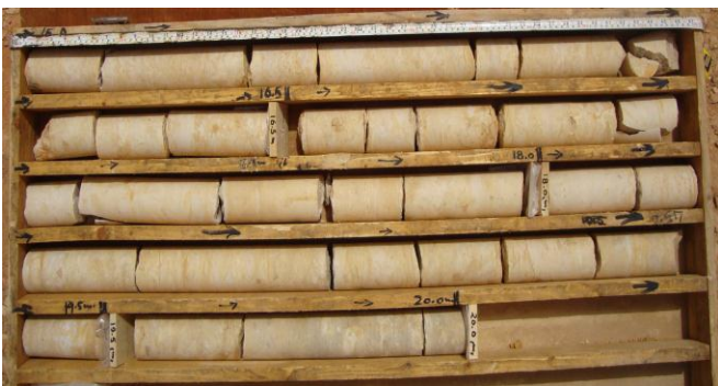
Photo 1. Represent the Core samples from one borehole
