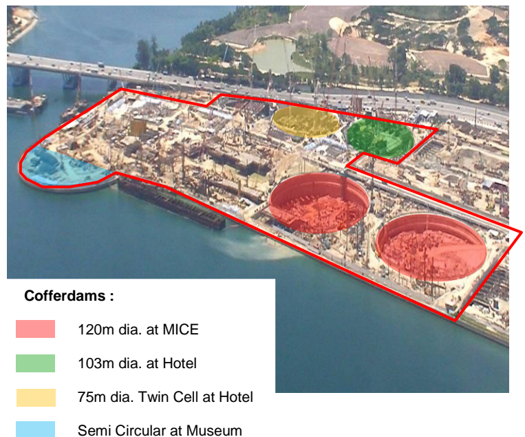
Fig. 4. Excavation plan and location of circular cofferdams.
