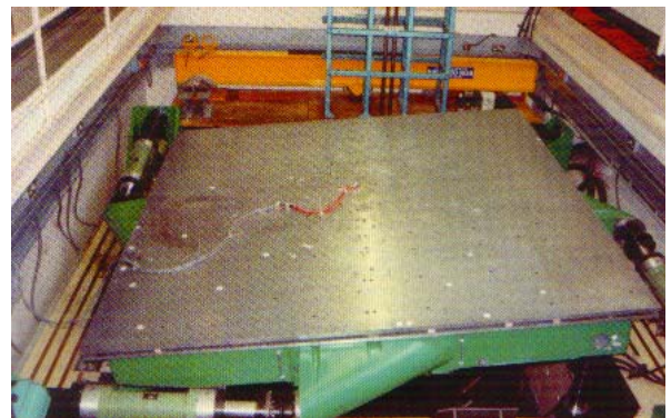
Fig. 5. Shaking table used for the experimental analysis.
