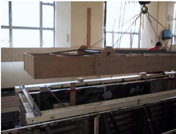
Fig. 2. Sieve for the deposition of the Leighton Buzzard sand into the shear stack.
