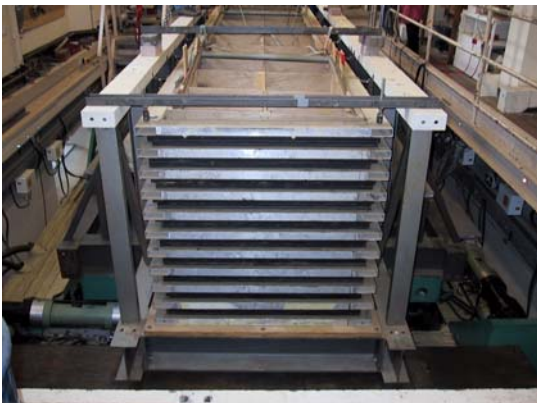
Fig. 3. Shear stack: short side [Biondi e Massimino, 2002].
