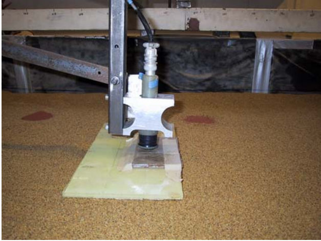
Fig. 10. The Ind26 displacement transducers.
