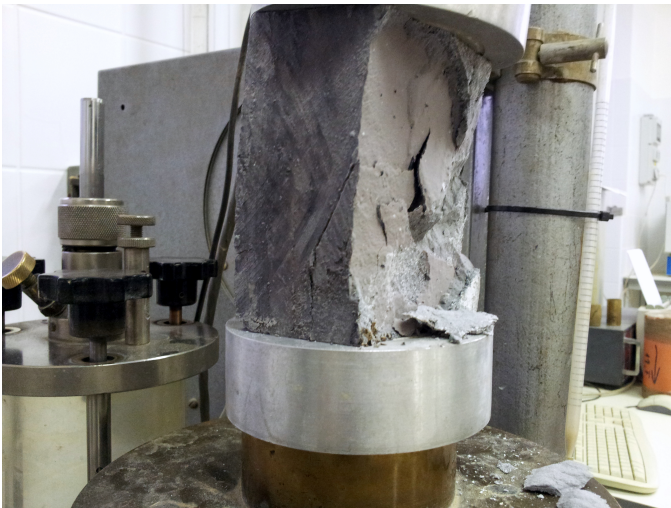
Fig. 11. Unconfined compression test
