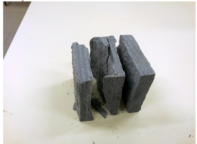
Fig. 10. Cracked dam sample
