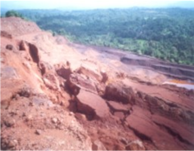
Pit Wall Collapse: Saniem Iron Ore Mine
