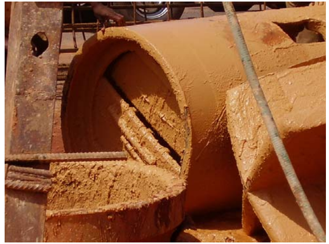
Fig.8 Close up view of chisel and bailer
