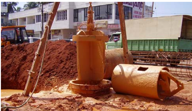
Fig. 7 Chisel and bailer for bored piles
