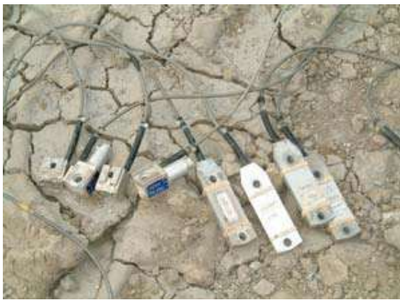
Fig. 38. Transducers and accelerometers
