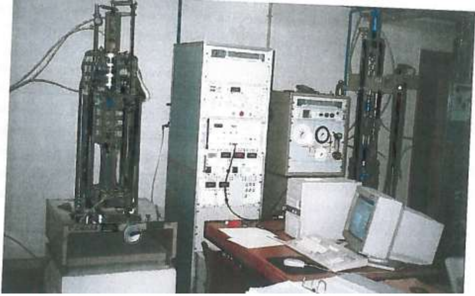
Fig. 13. View of cyclic torsional shear apparatus (after IST, 2005)
