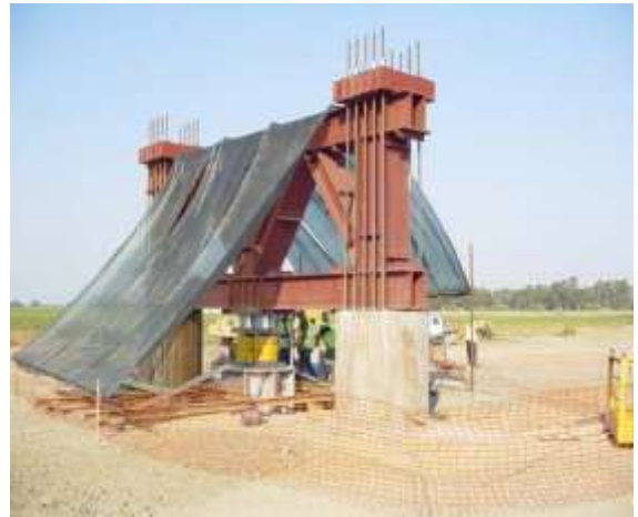
Fig. 33. General view for vertical pile load tests (after Ferreira et al, 2008)
