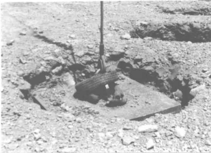
Fig. 6 - 15-ton, 900 psf tamper in crater after two drops
