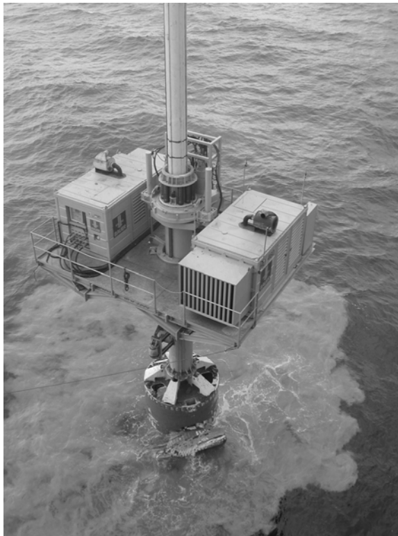
Fig. 20. Flydrill BFD 5500 with KB 3000 dumping drill spoil
