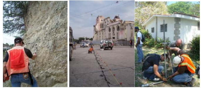
Fig. 1. Field activities in Haiti: geologic and damage mapping, MASW testing, and DCPT testing.
