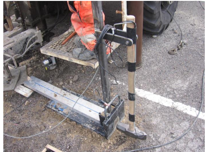
Fig. 6. L plate and sledge hammer for S waves generation.
